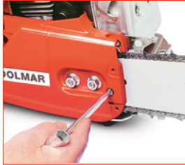
Lateral chain tensioning
