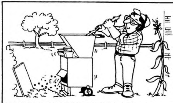
Use stick, never hands, if material bridges in hopper. Do keep people away and discharge shredded material into compost heap or fixed obstruction.
