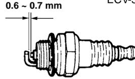
Clean the electrodes with a wire brush and reset the gap to 0.65 mm as necessary.
