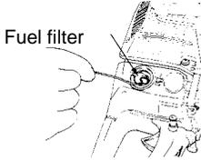
(b) Disassemble the filter and wash with gasoline, or replace with a new one if needed.
