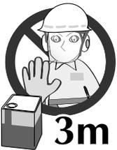
5. Always use caution when handling fuel. Wipe up all spills and then move the chain saw at least 3 m from the fueling point before starting the engine.
