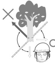
9. Never start cutting until you have a clear work area, secure footing, and a planned retreat path from the falling tree.
