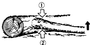
First check to which side the limb is bent. Then make the initial cut from the bent side and finish by sawing from the opposite side.
