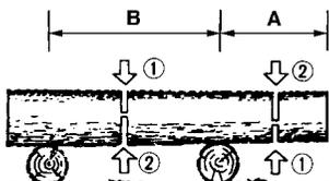
In area A, saw up from the bottom one-third and finish by sawing down from the top. In area B, saw down from the top one-third and finish by sawing up from the bottom.
