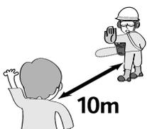
8. Do not allow other persons to be near the chain saw when starting or cutting. Keep bystanders and animals out of the work area. Children, pets and bystanders should be a minimum of 10 m away when you start or operate the chain saw.
