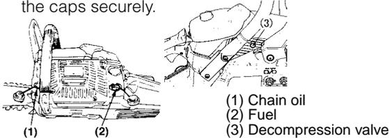
2. Set the switch to "I" position. Press the decompression valve (3).
