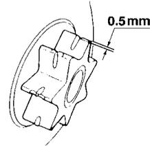
Check for cracks and for excessive wear interfering with the chain drive. If the wear is considerable, replace it with new one. Never fit a new chain on a worn sprocket, or a worn chain on a new sprocket.
