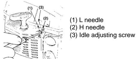
The carburetor on your unit has been factory adjusted, but may require fine tuning due to a change in operating conditions.
