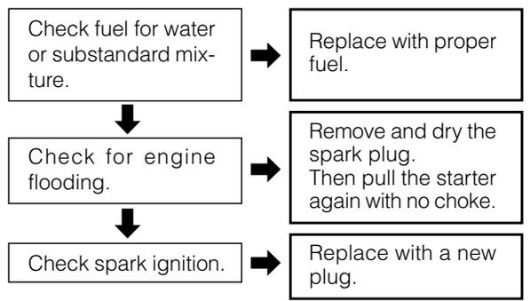
**Case 2. Lack of power/Poor acceleration/Rough idling**
