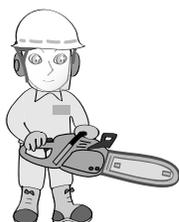
25. Guard against kickback. Kickback is the upward motion of the guide bar which occurs when the saw chain at the nose of the guide bar contacts an object. Kickback can lead to dangerous loss of control of the chain saw.
