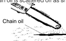
The chain oil flow can be changed by inserting a screwdriver in the hole on bottom of the clutch side. Adjust according to your work conditions.
