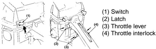
3. While holding the throttle lever together with the throttle interlock, push in the side latch and release the throttle lever to hold it at the starting position.
