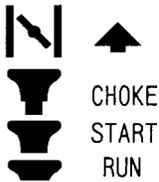
Starting the engine. If you pull out the choke knob (at the back-right of the rear handle) to the point of the arrow, you can set the starting mode as follows:
